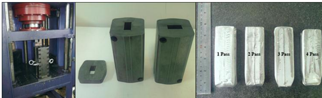
Figure 2. The hydraulic press, ECFE die parts (entrance channel, MDZ and exit channel), and CP aluminum billets after the ECFE process up to the four passes.
