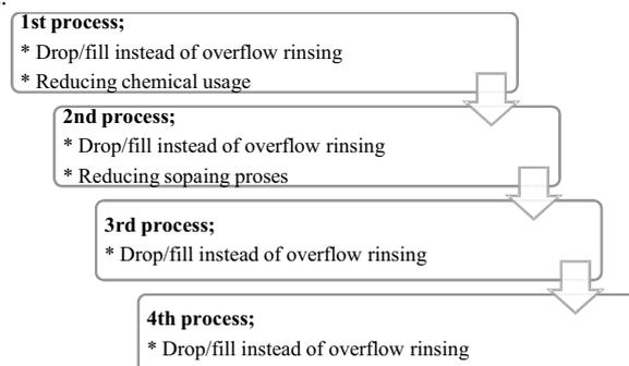
Fig 2. Processes applied to obtain water savings
