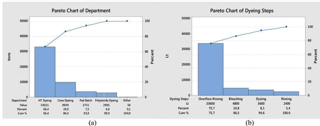
Fig 1. Minitab Pareto analysis results (a) for water consumption ratios of dye house departments,(b) for water consumption ratios of reactive dyeing process
