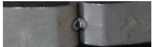
Fig. 5. Knotting failure observed in weld nuggets.
