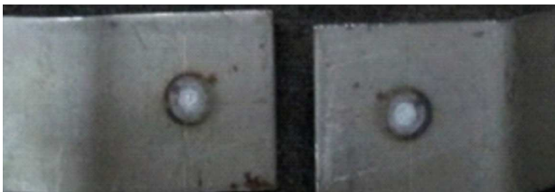
Fig. 3. Separation failure observed in weld nuggets.
