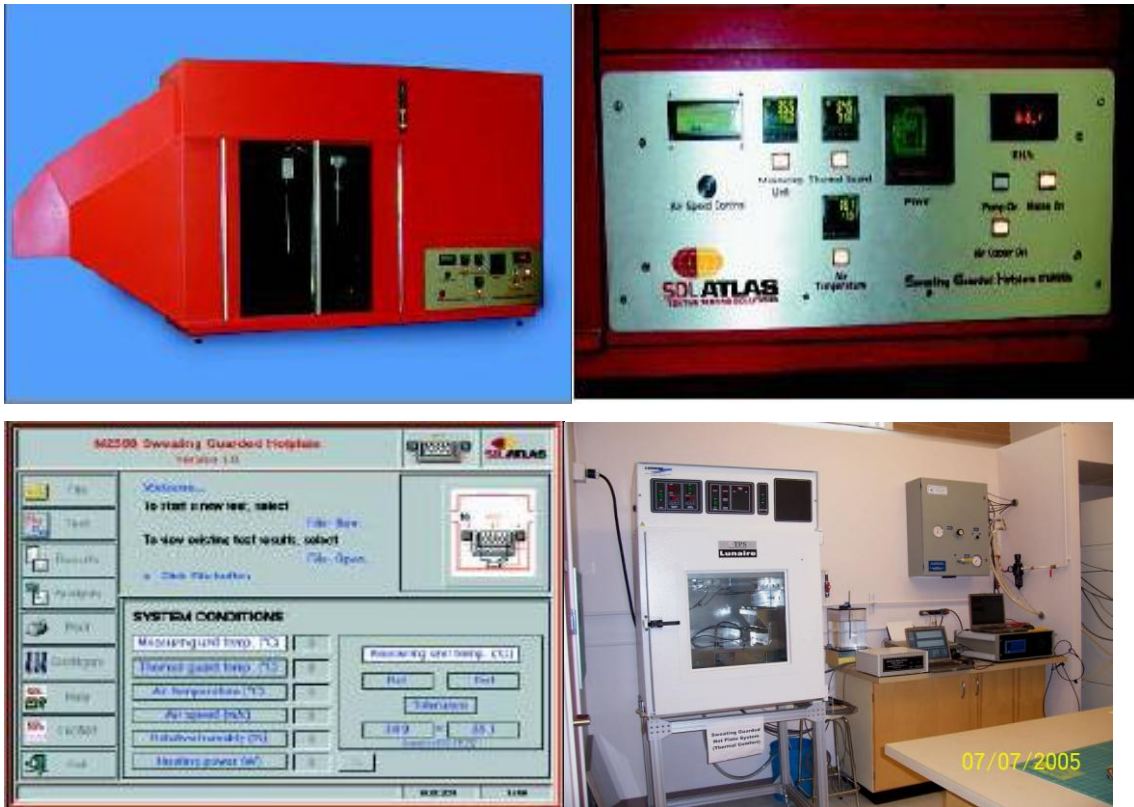
Şekil 2.15 Sweating guarded hot plate (WEB_8 2007)
