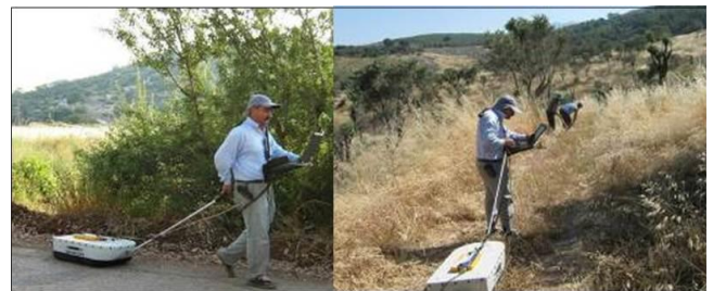
Figure 4: GPR profile measurements in the field.
