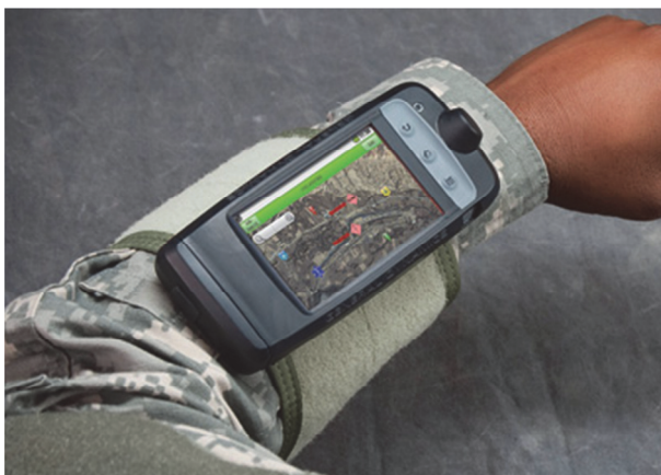
Figure 4.6.5 A PDA tied up to the arm of a Soldier (Source: ISSSP-International Strategic and Security Studies Programme, http://issp.in/wearable-military-technologies/ )
