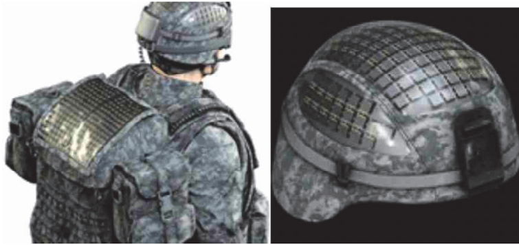
Figure 4.6.2 (a) Soldier backpack with flexible solar cells,( b) Flexible Solar energy harvesters in helmets
