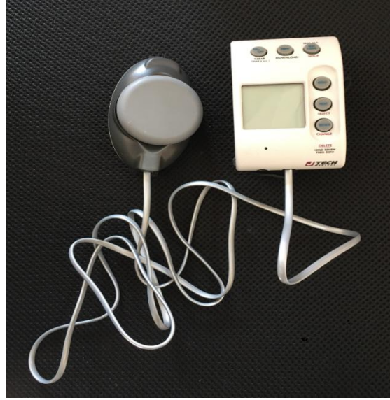
Resim 3.5.2.3.1 Hand-held Dinamometre (HHD) (Commander Power Track II; JTECH Medical Industries, Salt Lake City, UT).
