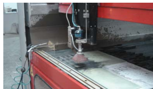
Fig. 3: Specimen cutting with using water jet.
