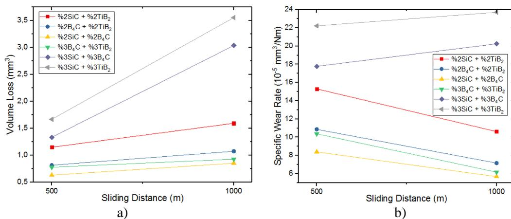
**Fig. 4.** (a) Volume loss and (b) specific wear rate of Al 7075 hybrid composites.
