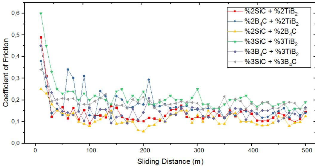
Fig. 5. Coefficient of friction of Al 7075 composites.
