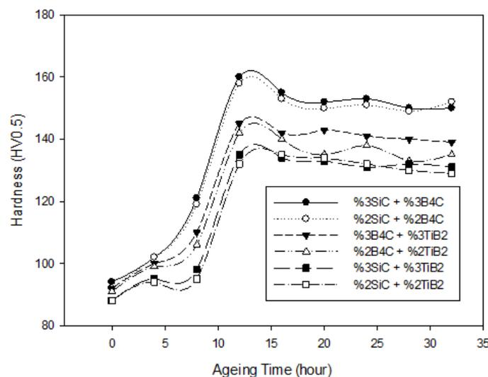
**Fig. 3.** Hardness values of Al 7075 + B<sub>4</sub>C/SiC/TiB<sub>2</sub> hybrid composites after aging.
