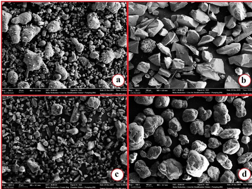
**Fig. 2.** Field emission SEM images of powders used in the study: (a) Al 7075, (b) SiC, (c) B<sub>4</sub>C, (d) TiB<sub>2</sub>.
