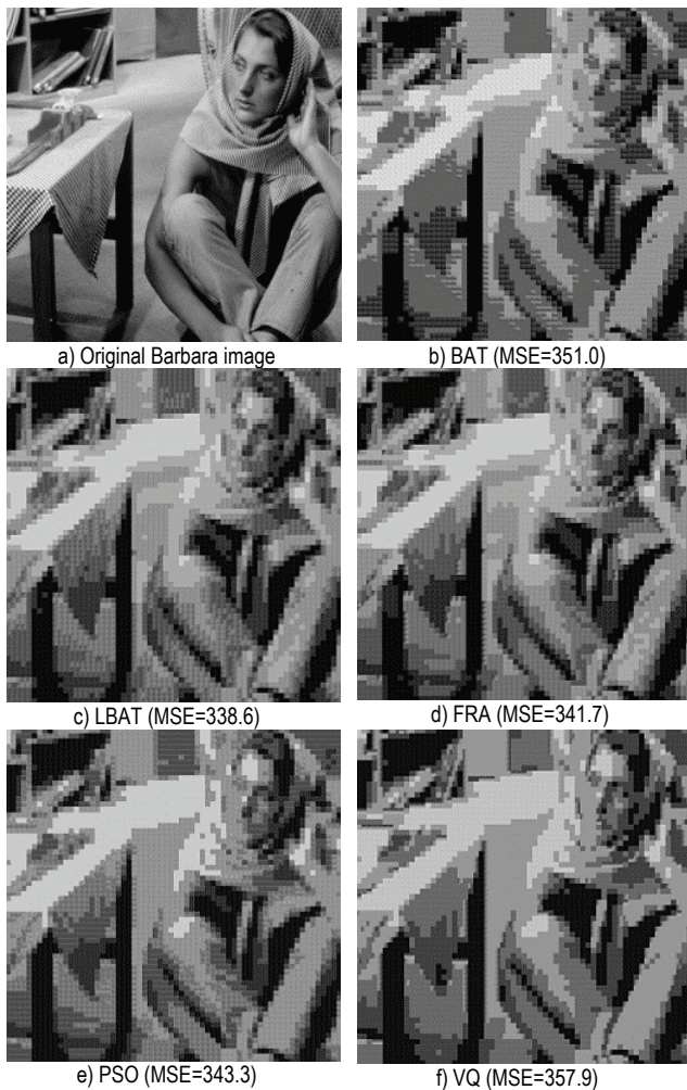
Figure 4 Visual results of LBAT, BAT, FRA, PSO and VQ algorithms for BARBARA image for 8 codewords of codebook
