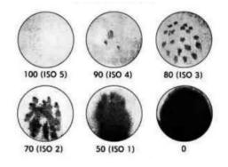
*Figure 1: Rating Marks according to AATCC test method*
