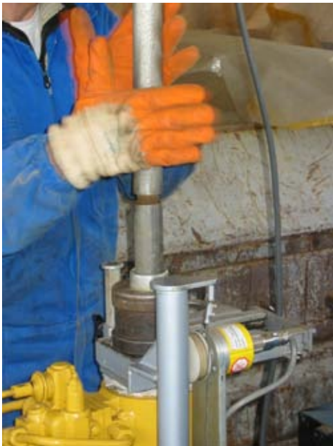
c) Connecting thrust rods to ER-VPT tool
