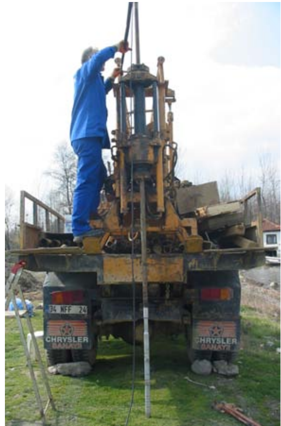
b) ER-VPT instrument pushed into the ground
