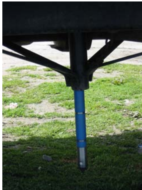
d) ER-VPT instrument pushed into the ground
