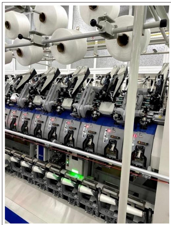
Figure 1. Image of core-spun vortex yarn production on MVS 870 spinning machine (Original image captured in Karafiber Textile Company).
