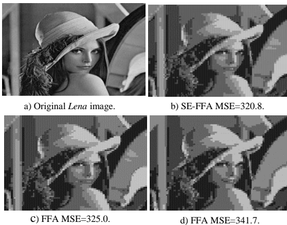
Figure 9. a) Original 256x256 pixel size of high contrast Lena image with COV=0.530. b) Proposed SE-FFA with MSE=320.8. c) Classical FFA result with MSE=325.0 d) Classical FFA result with MSE=341.7 the radius is selected as 2 pixels, compression ratio is selected as 0.122 bpp.
