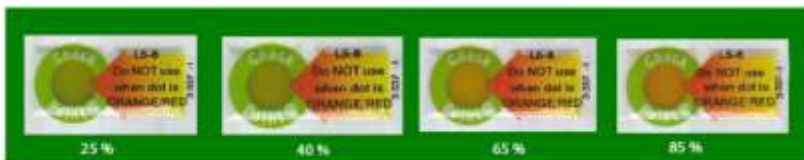
Figure 11. Enzymatic based time-temperature indicators (Öcal and Çakmak Karapınar, 2016).
