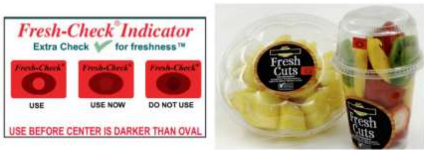
Figure 12. The Fresh-Check® TTI label (Fresh-check is a registered brand of the TEMPTIME Corporation, Morris Plains, NJ, USA) of which the color of the inner circle changes (depending on time and temperature) and needs to be compared to the outer circle to establish use-by status.
