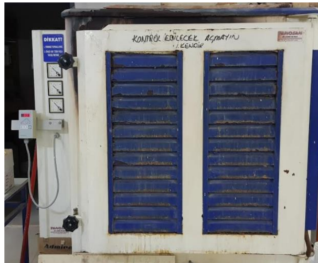
Figure 2. Ceramic furnace used in experiments
