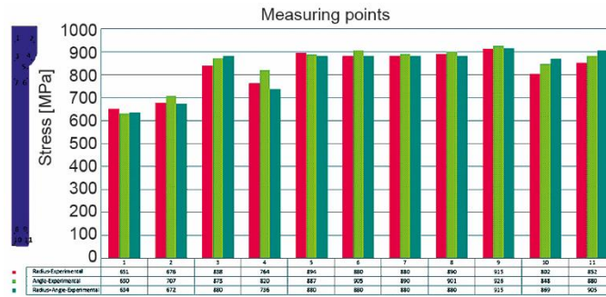
Figure 7. Experimental and numerical analysis of the data obtained according to the hardness measurement zones in the radius-angle mold sample (for color image see journal web site)
