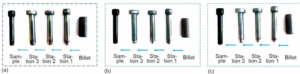
Figure 3. Processing steps of samples produced according to different extrusion die-sample forms; (a) radius extrusion die, (b) angled extrusion die, and (c) radius and angled extrusion die
