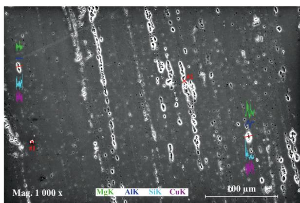
Figure 5: Line EDS and point EDS measurements from TMAZ
