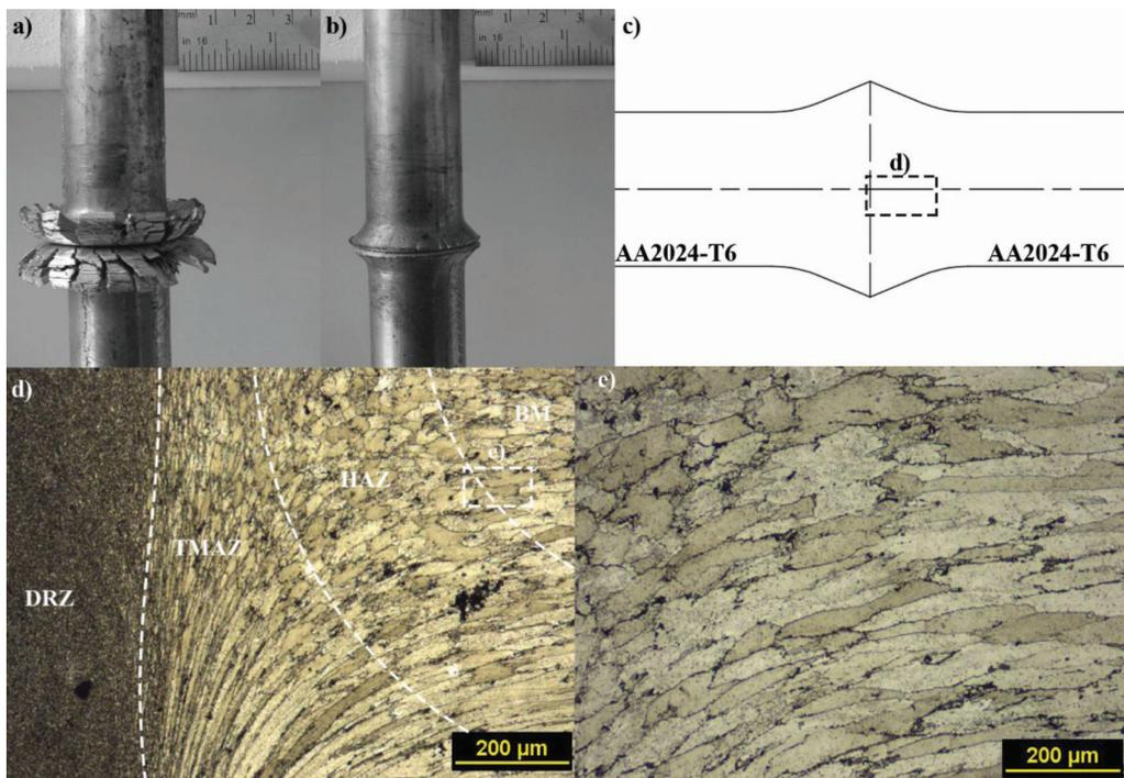
**Figure 3:** Macro image of a) untrimmed and b) trimmed rotary-friction specimen, c) schematic of the LOM image, microstructure image from d) cross-section and e) HAZ and BM interface
