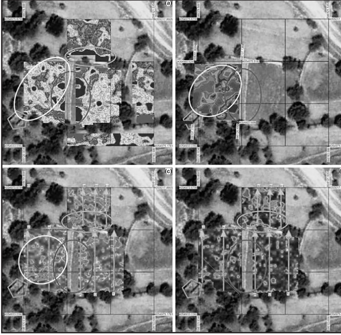
Figure 10: Comparison of the results of the integrated geophysical studies carried out in the north of the sanctuary. (a) Magnetic gradiometer (b) ERT depth slice (0-0.375 m), (c) georadar depth slice (0-0.5 m), (d) georadar depth slice (0.5-1.5 m) (PAP archive).
