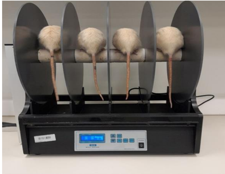
Figure 3.7. Motor performance measurement using rotarod apparatus.
