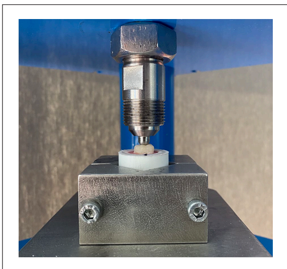
Figure 2. Mounted specimen in the universal testing machine.
