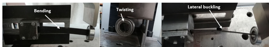
FIGURE 8 Laterally buckled specimen.
