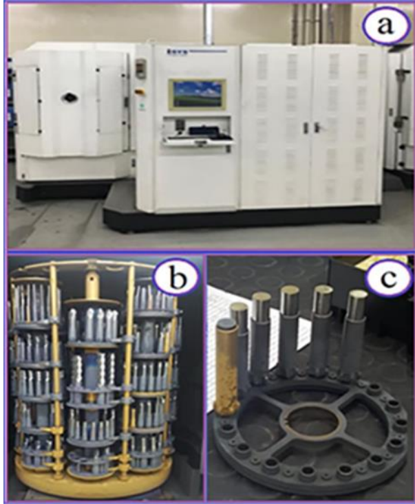
Figure 1. a) PVD coating machine (ISYS Intelligent System 190A), b), c) The specimens were placed in the coating boxes
