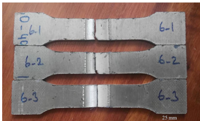
FIGURE 9 Photograph of the samples joined at 1250 rpm 400 \text{ mm}\cdot\text{min}^{-1} parameter after the tensile test. 1 [Colour figure can be viewed at wileyonlinelibrary.com ]
