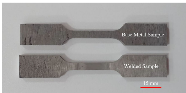
FIGURE 6 Base metal and welded fatigue test specimens. 1 [Colour figure can be viewed at wileyonlinelibrary.com ]
