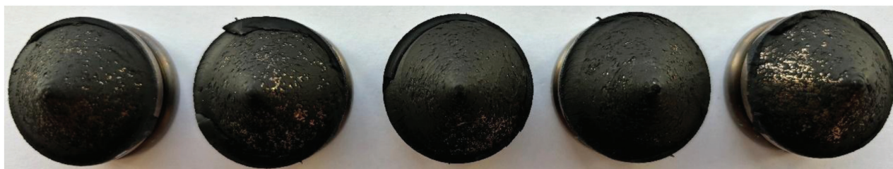
Figure 2: Surface images of the specimens tested by Method C of ASTM D429-14 standard
