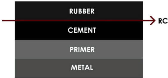
Figure 5: Rubber-Cover Cement interface failure
