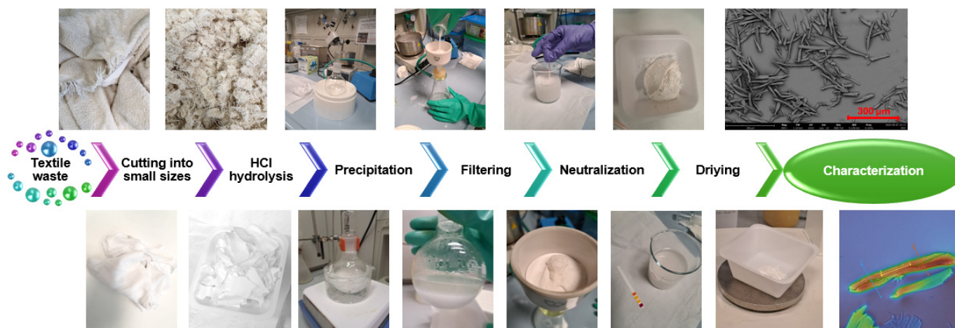
Figure 1. MCC production process.
