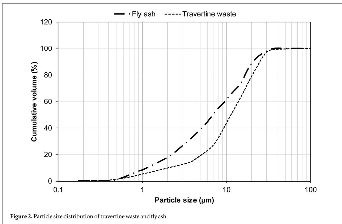
Figure 2. Particle size distribution of travertine waste and fly ash.
