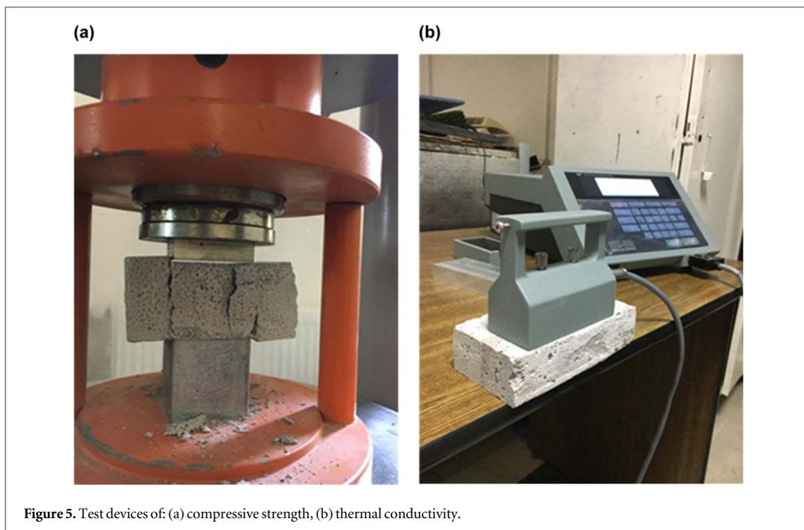
**Figure 5.** Test devices of: (a) compressive strength, (b) thermal conductivity.
