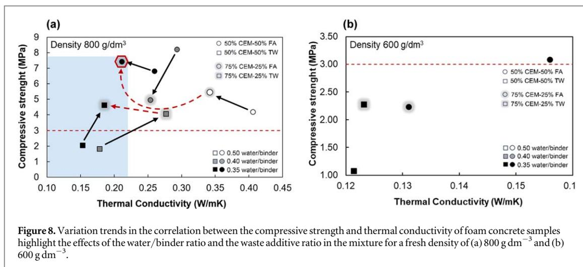
**Figure 8.** Variation trends in the correlation between the compressive strength and thermal conductivity of foam concrete samples highlight the effects of the water/binder ratio and the waste additive ratio in the mixture for a fresh density of (a)  $800 \text{ g dm}^{-3}$  and (b)  $600 \text{ g dm}^{-3}$ .
