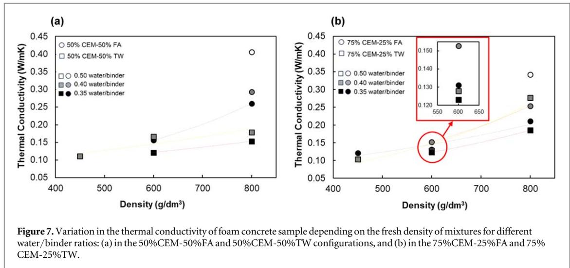
**Figure 7.** Variation in the thermal conductivity of foam concrete sample depending on the fresh density of mixtures for different water/binder ratios: (a) in the 50%CEM-50%FA and 50%CEM-50%TW configurations, and (b) in the 75%CEM-25%FA and 75%CEM-25%TW.
