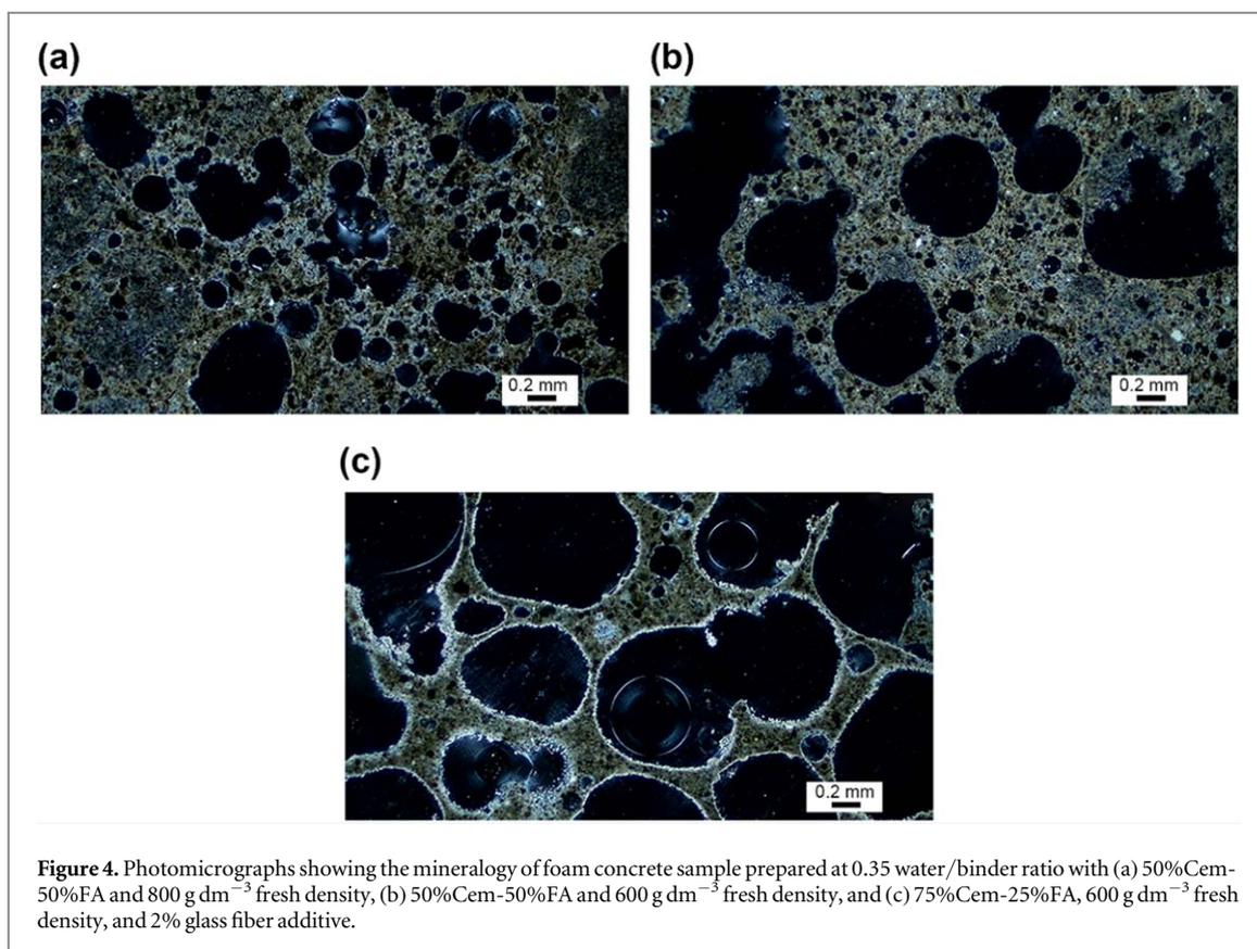
**Figure 4.** Photomicrographs showing the mineralogy of foam concrete sample prepared at 0.35 water/binder ratio with (a) 50% Cem-50% FA and 800 g dm<sup>-3</sup> fresh density, (b) 50% Cem-50% FA and 600 g dm<sup>-3</sup> fresh density, and (c) 75% Cem-25% FA, 600 g dm<sup>-3</sup> fresh density, and 2% glass fiber additive.
