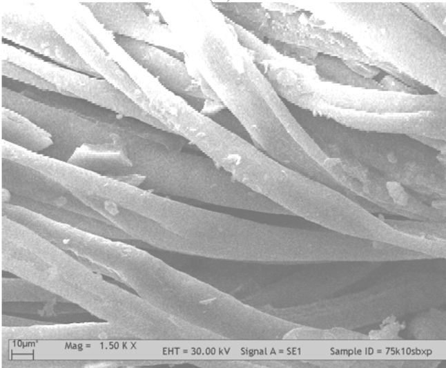
Figure 1. SEM micrographs of (a) untreated fabric, (b) fabric treated with fire retardant solution R17, (c) fabric treated with fire retardant solution R17 and 5 times washed, (d) fabric treated with fire retardant solution R12, (e) fabric treated with fire retardant solution R12 and 5 times washed.
