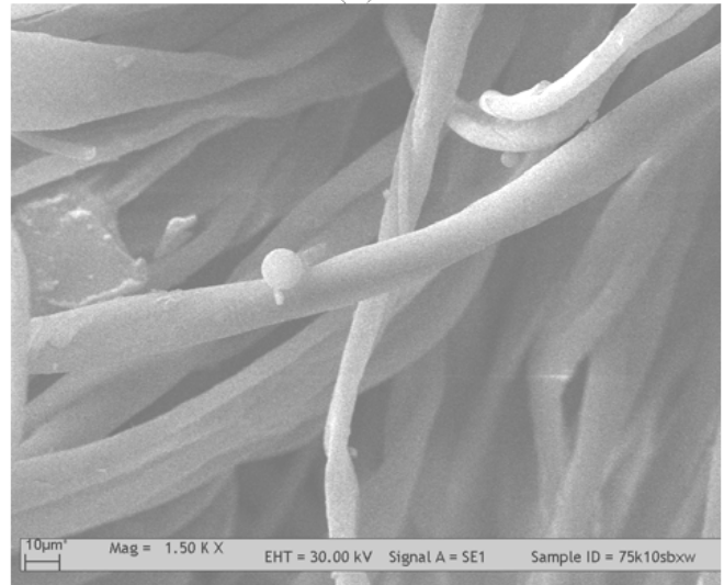
Figure 1. SEM micrographs of (a) untreated fabric, (b) fabric treated with fire retardant solution R17, (c) fabric treated with fire retardant solution R17 and 5 times washed, (d) fabric treated with fire retardant solution R12, (e) fabric treated with fire retardant solution R12 and 5 times washed.
