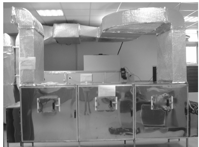
FIG. 1. (a) Schematic of the heat pump dryer with coded points used in equations; (b) Picture of the heat pump dryer.
