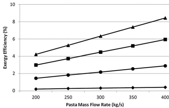
Figure 5. Variation of exergy efficiencies with mass flow rates of pasta for each dryer;  $\blacktriangle$  predryer,  $\blacksquare$  first dryer,  $\bullet$  second dryer, and  $\blacklozenge$  third dryer.
