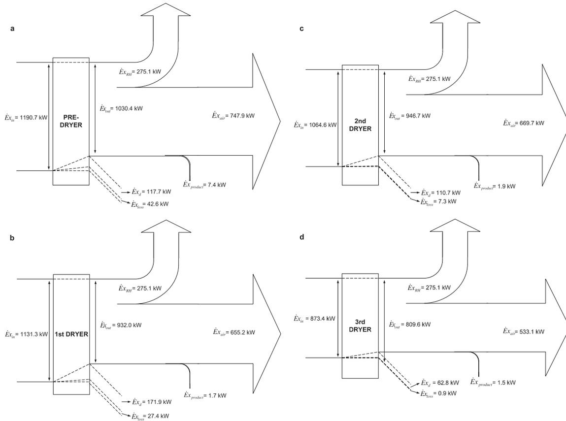
Figure 3. Exergy loss, destruction, and flow diagram (Grassmann diagram) for the pasta-drying system for each dryer; (a) predryer, (b) first dryer, (c) second dryer, and (d) third dryer.
