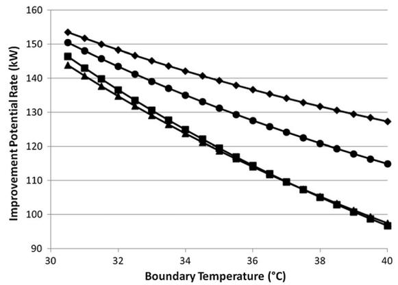
Figure 8. Variation of improvement in potential rates with different boundary temperatures for each dryer;  $\blacktriangle$  predryer,  $\blacksquare$  first dryer,  $\bullet$  second dryer, and  $\blacklozenge$  third dryer.
