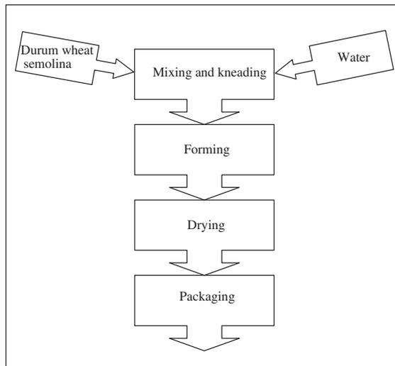
Figure 1. Flow diagram of pasta production.
