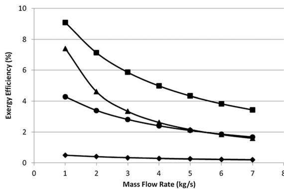
Figure 6. Variation of exergy efficiencies with mass flow rates of drying air for each dryer;  $\blacktriangle$  predryer,  $\blacksquare$  first dryer,  $\bullet$  second dryer, and  $\blacklozenge$  third dryer.
