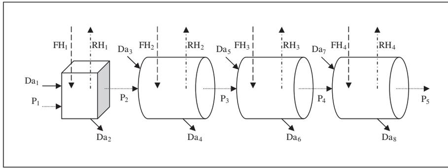
Figure 2. Schematic illustration of a four-step industrial farfalle pasta-drying system.
