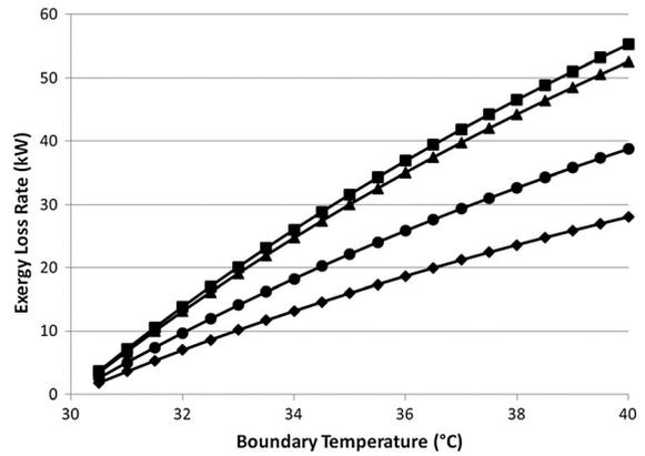
Figure 7. Variation of exergy loss rates with different boundary temperatures for each dryer;  $\blacktriangle$  predryer,  $\blacksquare$  first dryer,  $\bullet$  second dryer, and  $\blacklozenge$  third dryer.
