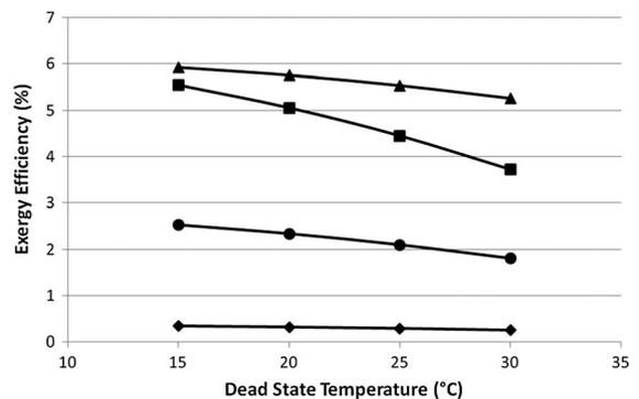
Figure 9. Variation of exergy efficiencies with dead state temperature for each dryer;  $\blacktriangle$  predryer,  $\blacksquare$  first dryer,  $\bullet$  second dryer, and  $\blacklozenge$  third dryer.
