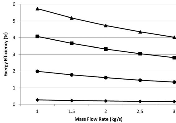
Figure 4. Variation of exergy efficiencies with mass flow rates of hot water for each dryer;  $\blacktriangle$  predryer,  $\blacksquare$  first dryer,  $\bullet$  second dryer, and  $\blacklozenge$  third dryer.
