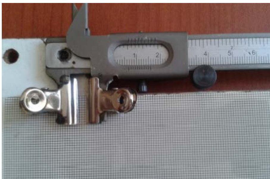
Figure 2. Designed jaw moving platform with millimeter ground fabrics used in the study.
