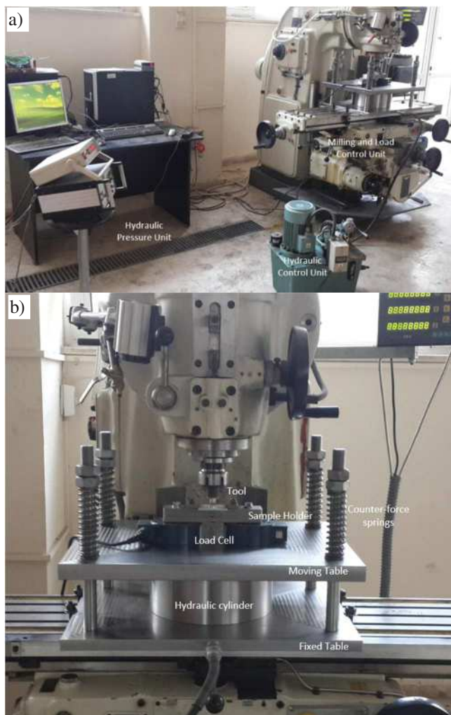
Fig. 2. The view of the experimental setup, a) (general), b) (fixing)
