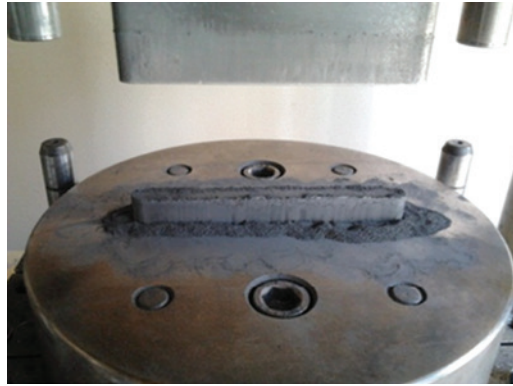
Figure 2 A beam sample after cold pressing.
